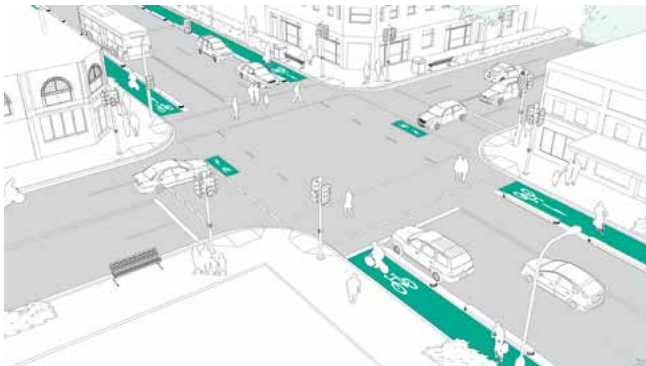
Figure 3.19 Bicycle path (one-way), signalised intersection - perspective
