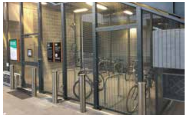
Figure 4.5 Bicycle sheds can be integrated seamlessly into station design and provide ample space for commuters for the first or last mile of their journey. They should be fully integrated with the Opal card system to enable ease of access. They should be located in an area of the station that has active (ie. CCTV) and passive (ie. regular passers-by) surveillance at all times, and that is well-lit
