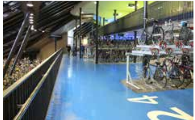
Figure 4.3 Bicycle hubs are the preferred parking facility for transport stations and interchanges where demand is high. They should be well signed, have level access, and be accompanied by complementary amenities like bathrooms, tyre pumps, tool kits, showers and change rooms, as appropriate
