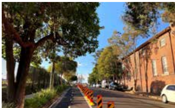
Figure 6.5 Two-way cycle facilities require less street space and may require changes to signalised intersections
