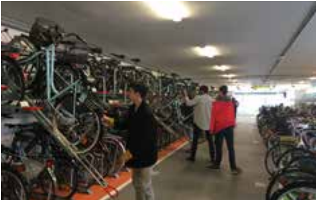
Figure 4.2 Bicycle parking can be stacked for efficient use of space, and should be provided in high-quality, sheltered hubs with good lighting and active surveillance
