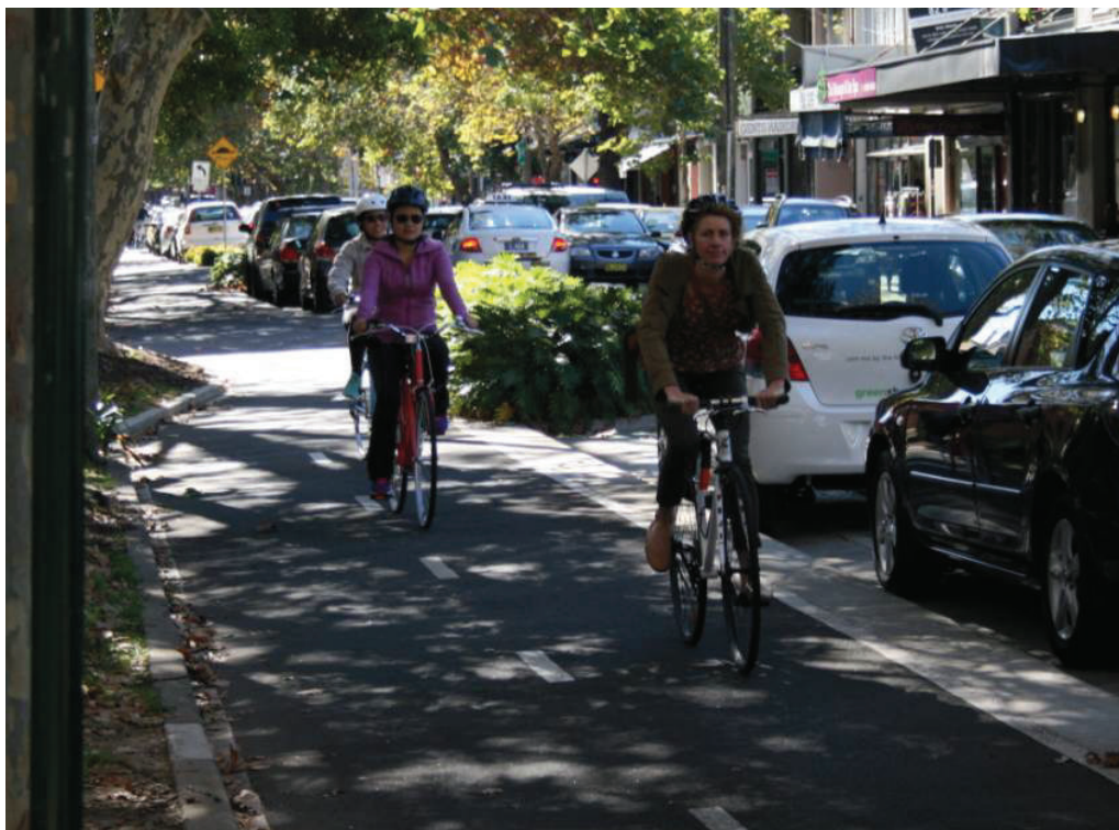
Figure 72: Two way cycle track diverted to retain street tree, Bourke St, Sydney
