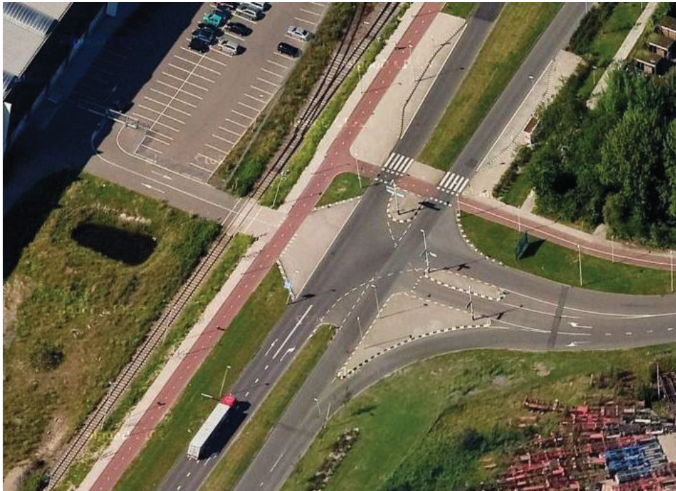
Figure 69: Industrial area driveway crossing two-way cycle track, Rotterdam
