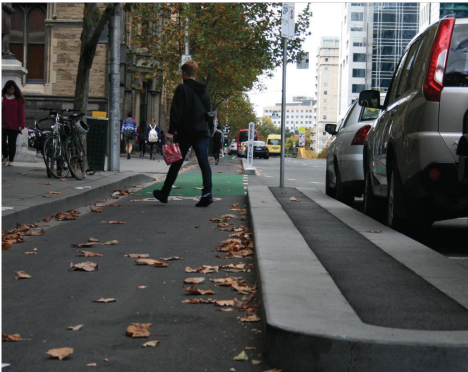
Figure 23: One-way cycle track on 2-way multilane road, median separated profile, Latrobe St, Melbourne. This example shows 1.1 m median with parking and further down a 0.3 m median where there is no parking
