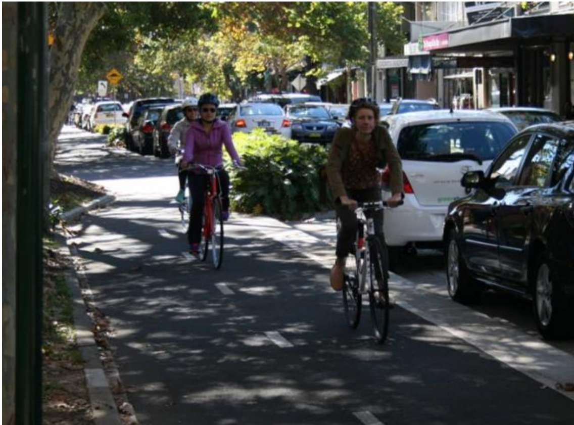
Figure 3.3.5(B) – Two-way cycle track diverted to retain street tree, Bourke Street, Sydney
