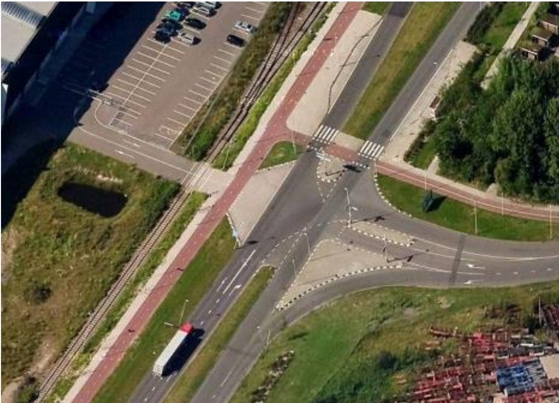
Figure 4.7.2(B) – Two-way cycle track crossing industrial area driveway, Rotterdam
