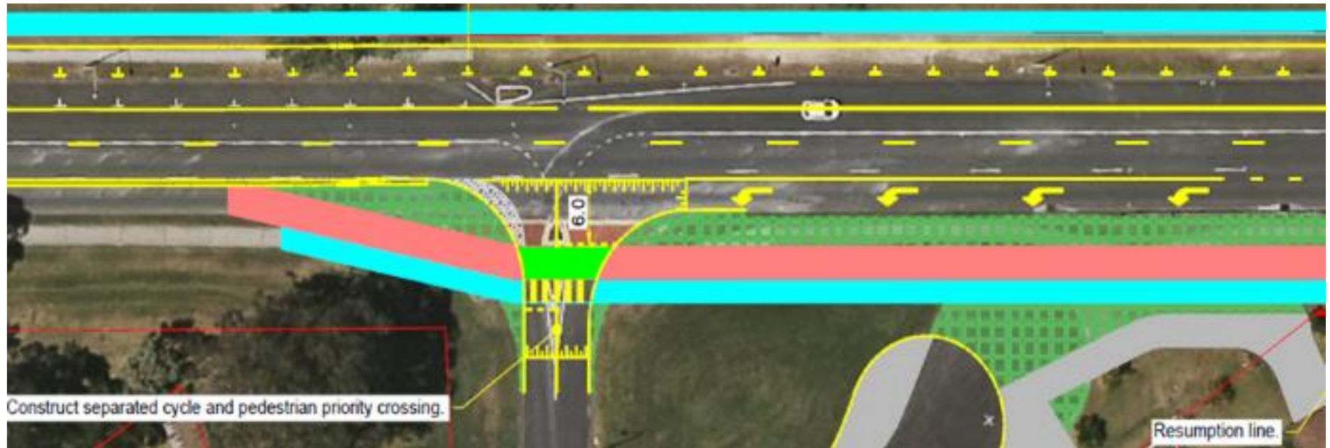
Figure 4.3.1(C) – Concept drawing of two-way cycle track with 6 m storage for exiting vehicles and 3 m buffer for vehicles entering from the added left-turn lane (LTS2)
