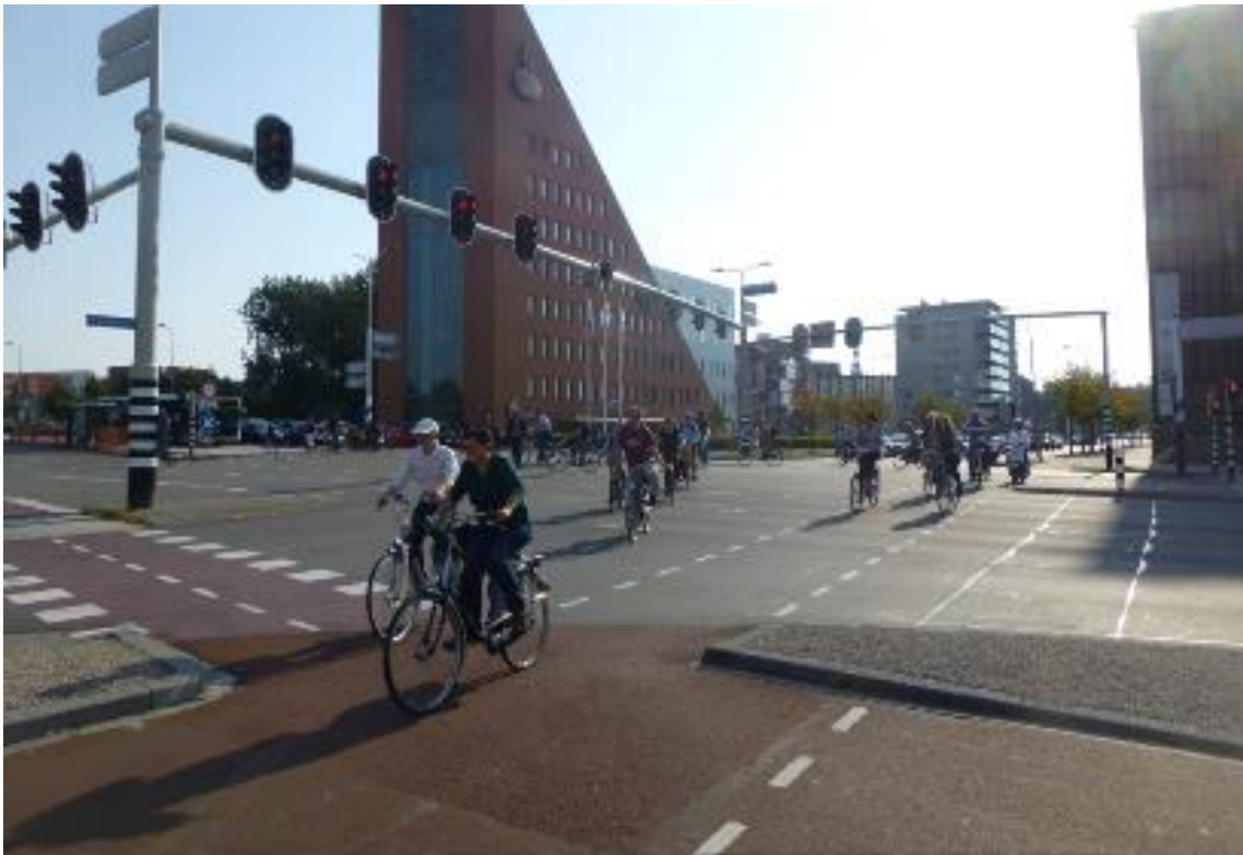
Figure 4.5.2(L) – All directions green for bicycle traffic at a smaller intersection, Assen, The Netherlands
