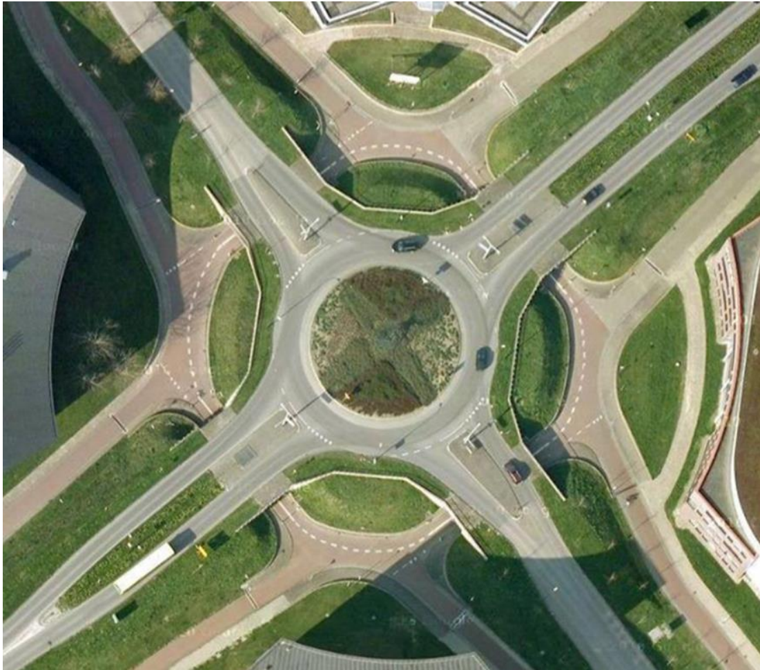
Figure 4.4.2(B) – The ultimate safe solution: pedestrian and bicycle underpasses for grade-separation at a single-lane roundabout, Houten, Netherlands (LTS1)
