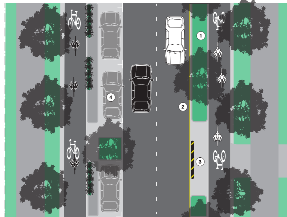
Two x 1-way separated cycle track with parking one side (preferred)
