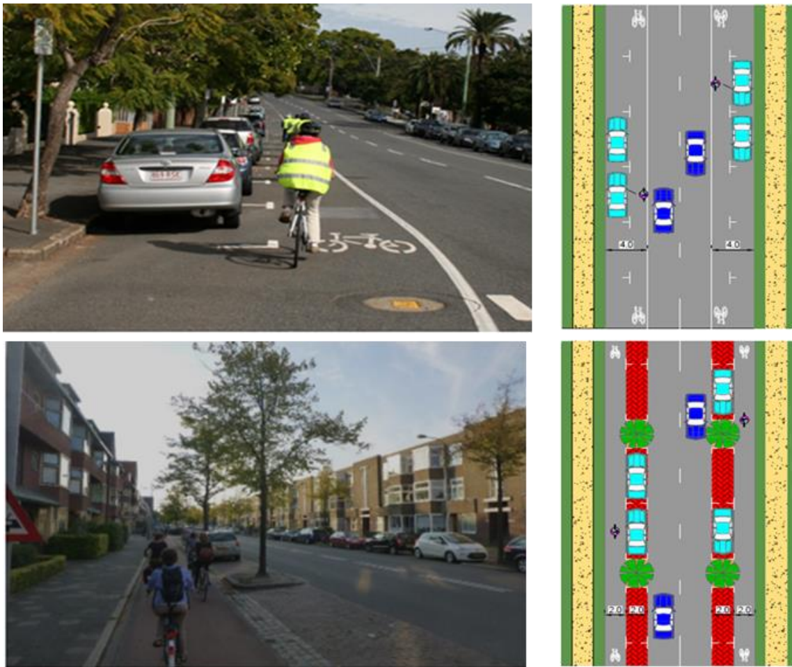
Figure 3.2.1.1(A) – Bicycle / car parking lane, Brisbane compared to one-way cycle track and parking, Assen, The Netherlands (both 4.0 m total width)
