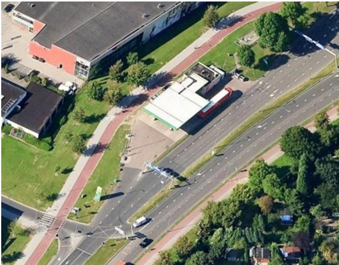
Figure 4.7.1 – Two-way cycle track and footpath on arterial road built behind the service station to avoid crossing conflicts, Rotterdam
