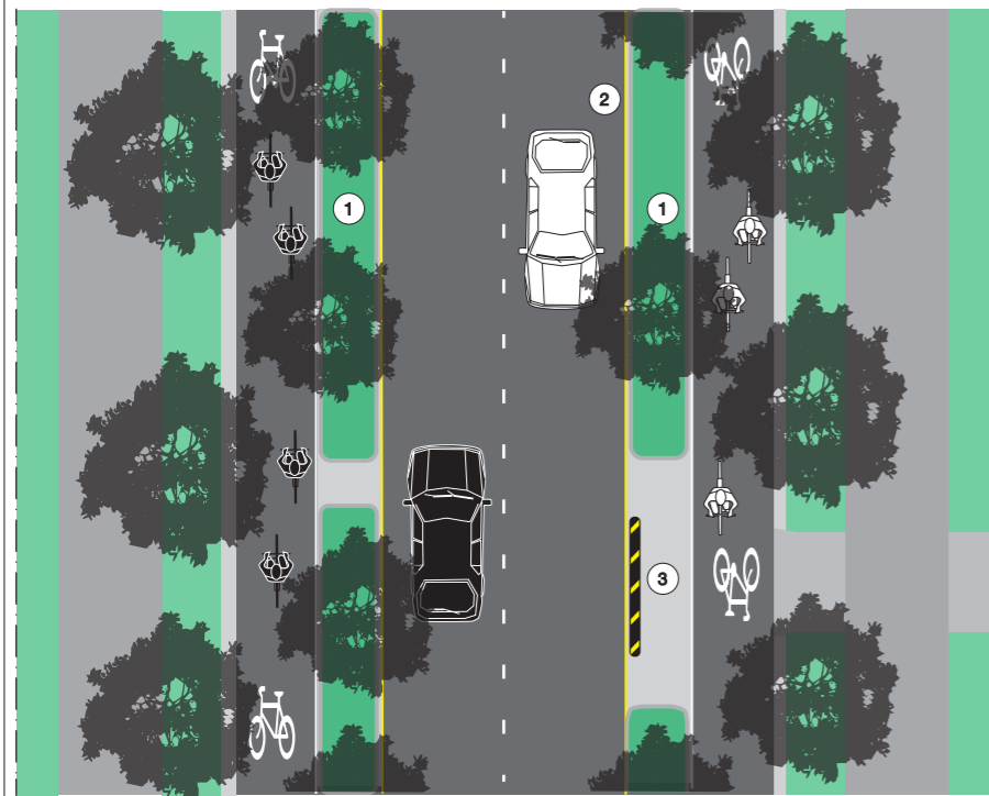
Two x 1-way separated cycle track (preferred)
