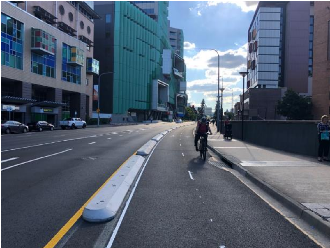
Figure 3.2.6.2(A) – Two-way cycle track, median separated profile, Woolloongabba, Brisbane
